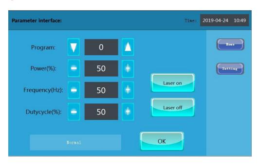
**Parameter serial number:** We can preset about 20 groups of welding parameters according to different materials. Just need to press the up and down button to choose the parameter.
