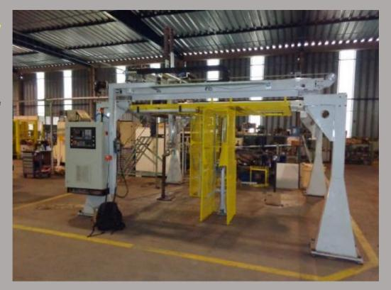
These gantry loaders also are full modular design and can be supplied to tend one or more machines with vertical arms moving on all X, Y and Z axis They can also have controls to allow their integration with other machines
